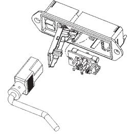
Figure 3. Power entry module door and fuse block.
