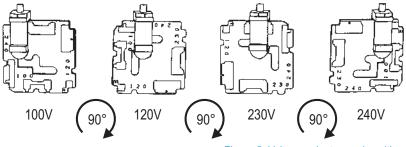
Figure 5. Voltage selector card positions.
