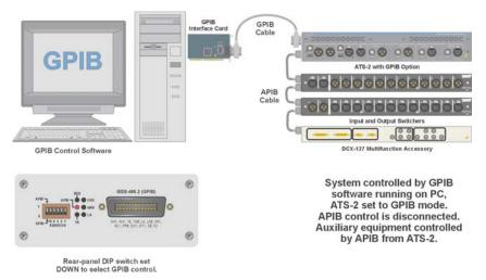
Figure 25. APIB connections to ATS-2 with GPIB option in GPIB control mode. SWR-2122 Switcher and DCX-127 connected to the APIB connector of the ATS-2. The computer APIB cable is not connected.
