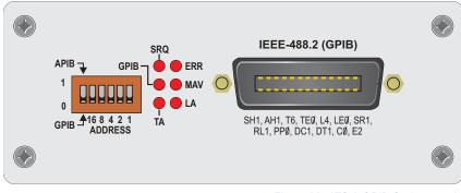
Figure 28. ATS-2 GPIB Option panel: Address Switch, Status LEDs and GPIB port.
