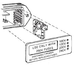
Figure 4. Changing the mains power supply voltage.
