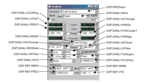
Figure 22. ATS-2 Audio Analyzer panel with GPIB command call-outs.
