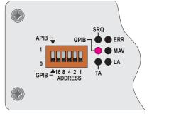
Figure 23. The ATS-2 Option GPIB panel; detail, shown in GPIB mode.
