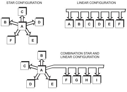
Figure 27. GPIB devices may be connected in star, linear, or combination star/linear configurations.
