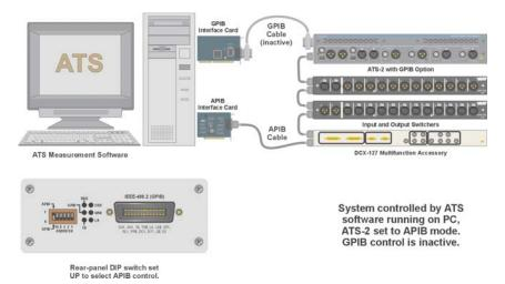
Figure 26. APIB controller connections, ATS-2 with GPIB option in APIB control mode. Computer APIB cable connected to DCX-127, then to SWR-2122, then to ATS-2.
