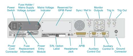
Figure 10. ATS-2 rear panel, APIB-only configuration.
