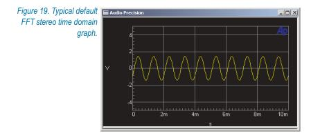
The display shows a sine wave with a period of 1 ms (corresponding to a frequency of 1 kHz) and a peak excursion of 1.414 V (corresponding to an amplitude of 1 Vrms). The effect of the distortion on the waveform is not visible in the time domain.
