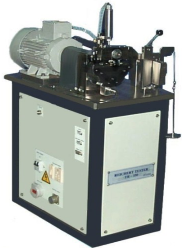
Reichert Tester by Ducom for lubricant performance testing.
