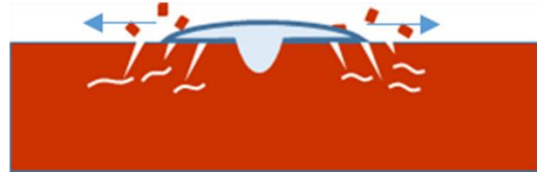
Figure 3. (a) In Phase II lateral jetting where water drop spreads outward with velocity 10 times greater than impact with generation of both shear and Rayleigh waves. (b) Rayleigh waves lead to shear damage or microcracking followed by water drop lateral spreading which removes surface asperities.
